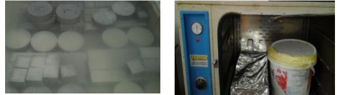
Specimens in normal water curing and hot water curing for 1-day
